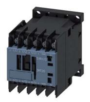
Power contactor, AC-3 9 A, 4 kW / 400 V 1 NO, 220 V AC, 50 Hz, 240 V 60 Hz, 3-pole, Size S00 ring cable lug connection
