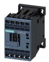
Power contactor, AC-3 9 A, 4 kW / 400 V 48 V AC, 50 / 60 Hz, 3-pole, Size S00 Spring-type terminal
