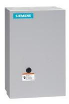
Electrically held lighting contactor, Contactor amp rating 100A, 0 N.C. / 3 N.O. Poles, 110VAC 50HZ/120VAC 60HZ coil, Non-combination type, (no disconnect device), Enclosure NEMA type 1, Indoor general purpose use
