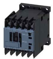
power contactor, AC-3 12 A, 5.5 kW / 400 V 1 NO, 100 V AC, 50 Hz 100-110 V, 60 Hz, 3-pole Size S00 ring cable lug connection
