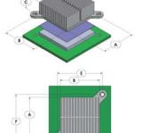
1) Dimension A is the length of the heat sink in the direction of the flow.
