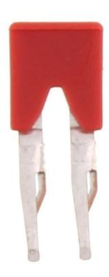
Insulated cross-connector, No. of poles: 2, Mounting type: Plug in, Width: 9.1 mm, Rated cross-section: 2.5 mm², Colour: Red
