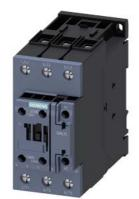
Power contactor, AC-3 80 A, 37 kW / 400 V 1 NO + 1 NC, 230 V AC, 50 Hz 3-pole, size S2 screw terminals
