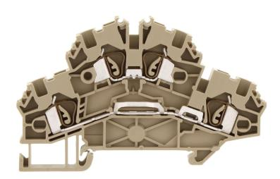
Double-level terminal, Tension-spring connection, Mounting type: Mounting rail TS 35/7.5, Rated cross-section: 2.5 mm², Width: 5.1 mm, Colour: Beige
