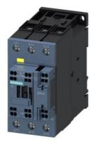
contactor, AC-3, 80 A/400 V/60  $^{\circ}\text{C}$  S2, 3-pole, 21-33 V AC/DC, F-PLC-IN, with varistor, 1 NC, spring-loaded terminal
