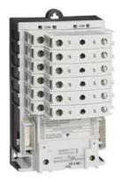
Electrically held lighting contactor, (convertible to mech. held), Amp rating 30A (tungsten 20A), 2 N.C. / 0 N.O. poles, 230-240V 60Hz/220V 50Hz coil, Non-combination type, Enclosure NEMA type (open), No enclosure
