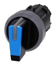
Selector switch, illuminable, 22 mm, round, plastic with metal front ring, blue, selector switch, short, 3 switch positions I-O<II, left latching, right momentary contact type, actuating angle  $2x45^{\circ}$ , 10:30h/12h/13:30h
