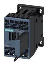
Traction contactor, AC-3 16 A, 7.5 kW / 400 V 24 V DC, 0.7-1.25\* Us with integrated varistor 3-pole, Size S00 Spring-type terminal
