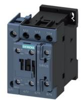
Contactor, AC-1, 35 A/400 V/40  $^\circ C,$  S0, 4-pole, 100 V AC/50 Hz, 110 V/60 Hz, 1 NO+1 NC, screw terminal
