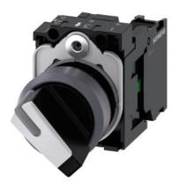
Selector switch, illuminable, 22 mm, round, plastic with metal front ring, white, selector switch, short, 2 switch positions O-I, latching, actuating angle 90°, 10:30h/13:30h, with holder, 1 NO, screw terminal, with laser labeling, upper case and lower case, always upper case at the beginning of the word
