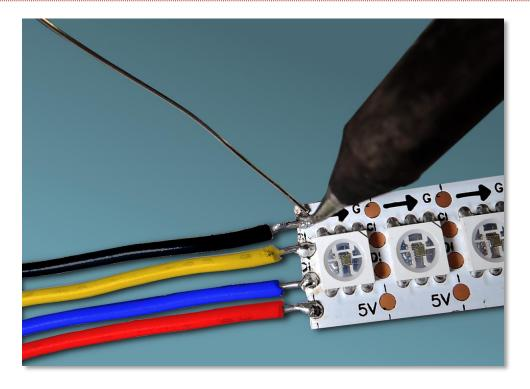
Ground (GND) and 5V are clearly marked on BrainPad's expansion header. As for C-Clock, it should connect to SCK on the BrainPad. D-Data should connect to MOSI on the BrainPad.
