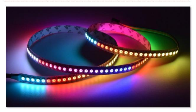
What you need to find are strips with the APA102 controller. This controller uses a SPI bus, which is available on the BrainPad. These strips are powered through different voltages. We will need 5V ones since we have access to 5V.
