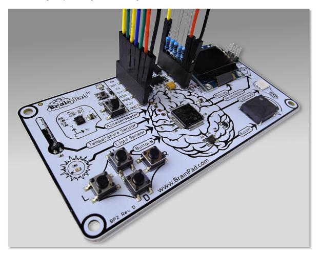
As mentioned in the first chapter of this book, there are multiple ways to expand the BrainPad, thanks to the female headers located near the USB connector.
