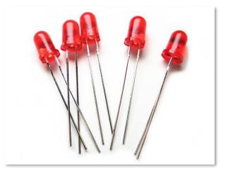
LEDs are very inexpensive and come in different colors. They have two leads where one should be longer than the other. Some LEDs have more than one color (like the BrainPad's Light Bulb.) We are not covering those LEDs. To control an LED a current-limiting resistor is needed. Some common values are 220, 330, or 470 ohms. You will also need some wires and a breadboard.
