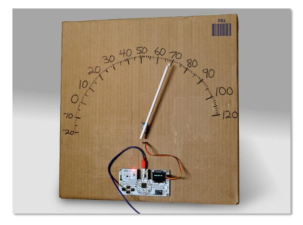
Here is finished thermometer made from a box and a straw glued to a servo motor.
