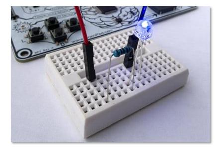
We can use one of the GPIO pins on the expansion header to control the LED. GPIO means General Purpose Input Output. We will use pin labeled PWM.
