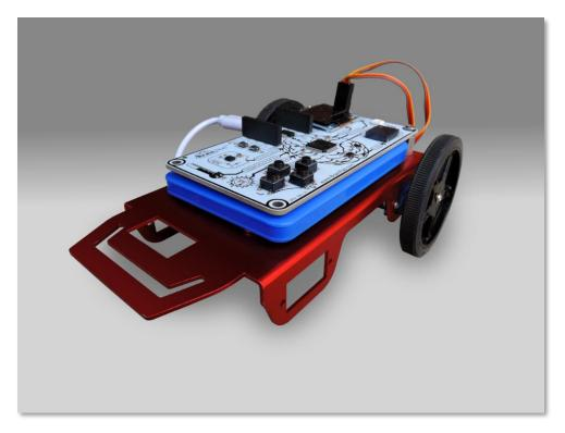
This robot is finally ready to dance! To go forward, both motors need to turn forward. However, as one of the motors is facing right and the other is facing left, one will have to turn opposite from the other for the wheels to
