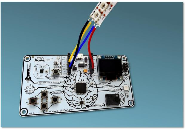
Each LED has three internal LEDs. They are red, blue and green. By controlling the levels of these base colors, you can create any color you wish. There are several online tools to help with color picking. A good example can be found at <u>http://www.rgbtool.com</u>. What you care about are the R, G, and B values.
