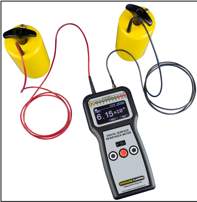
Figure 6. Electrical testing on the painted floor using a Surface Resistance Test Kit.
