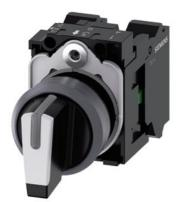
Selector switch, illuminable, 22 mm, round, plastic with metal front ring, white, selector switch, short, 3 switch positions I-O-II, latching, actuating angle  $2x45^{\circ}$ , 10:30h/12h/13:30h, with holder, 1 NO, 1 NO, spring-type terminal, with laser labeling, inscription or symbol Customer-specific selection with SIRIUS ACT configurator (CIN)
