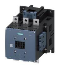
power contactor, AC-3 500 A, 250 kW / 400 V AC (50-60 Hz) / DC 21-27.3 V AC/DC auxiliary contacts 2 NO + 2 NC 3-pole, frame size S12 busbar connections drive: electronic with PLC interface 24 V DC spring-loaded terminal
