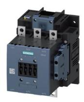
power contactor, AC-3 150 A, 75 kW / 400 V AC (50-60 Hz) / DC operation 96-127 V AC/DC auxiliary contacts 2 NO + 2 NC 3-pole, frame size S6 busbar connections drive: electronic with PLC interface 24 V DC screw terminal
