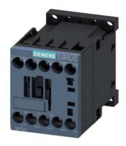
power contactor, AC-3 7 A, 3 kW / 400 V 1 NC, 24 V DC 0.7-1.25\* US, with diode integrated, 3-pole, size S00, screw terminal suitable for PLC outputs not expandable with auxiliary switch
