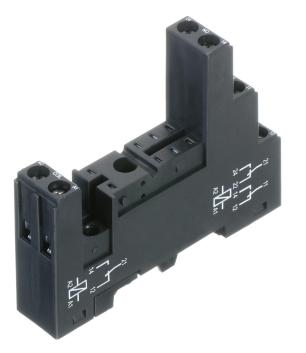
Relay socket base PRS, for miniature power relay with 2 CO contacts, Screw connection, Plug-in option for input/suppression modules, Mounting type: Mounting rail TS 35
