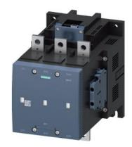
vacuum contactor, AC-3 400 A, 200 kW / 400 V AC (50-60 Hz) / DC operation 200-277 V AC/DC auxiliary contacts 2 NO + 2 NC 3-pole, frame size S12 busbar connections drive: electronic with SPS interface DV 24 V
