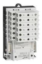
Electrically held lighting contactor, (convertible to mech. held), Amp rating 30A (tungsten 20A), 1 N.C. / 9 N.O. poles, 460-480V 60Hz/440V 50Hz coil, Non-combination type, Enclosure NEMA type (open), No enclosure
