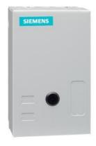
Electrically held lighting contactor, Contactor amp rating 30A, 0 N.C. / 4 N.O. Poles, 24VAC 50/60HZ coil, Non-combination type, (no disconnect device), Enclosure NEMA type 1, Indoor general purpose use
