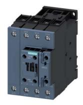
Contactor, AC-1, 110 A/400 V/40 °C, S2, 4-pole, 110 V AC/50 Hz, 120 V/60 Hz, 1 NO+1 NC, screw terminal
