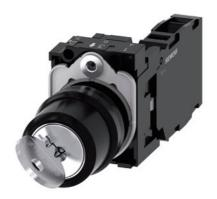
RONIS key-operated switch, 22 mm, round, plastic, lock number SB30, with 2 keys, 2 switch positions O-I, latching, 10:30h/13:30h, key removal O+I, with holder, 1 NO+1 NC, screw terminal, possible special locks: SB31, 421, 455, with laser labeling, lower case
