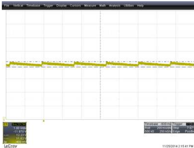
Figure 26. V_{OUT} , No Load, Aux Bias, Burst Interval is 340 ms, \Delta V_{OUT} is 400 mV
