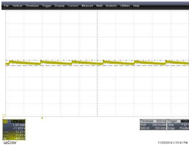
Figure 28. DC Coupled, V_{OUT} 0 A, Aux Bias Burst is Approximately 8-ms Long, Burst Rep Interval is Approximately 340 ms
