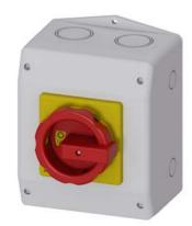
SENTRON, Switch disconnector 3LD, emergency switching-off switch, 3pole, lu: 63 A, operating power / at AC-23 A 400 V: 22 kW, Molded plastic encapsulation for inch cable gland, 1 NC, 1 NO, rotary operating mechanism, red/yellow
