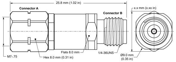
Figure 1. Product Dimensions for the ADP-2.4M-2.92F Adapter
