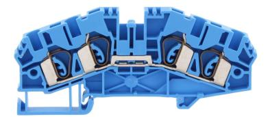
Ex feed-through terminal ATEX-certified, Tension-spring connection, Mounting type: Mounting rail TS 35/7.5, Rated cross-section: 4 mm<sup>2</sup>, Width: 6.1 mm, Colour: Blue
