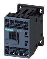
power contactor, AC-3 12 A, 5.5 kW / 400 V 1 NC, 24 V DC 0.7-1.25\*US 3-pole, size S00 spring-type terminal suitable for PLC outputs not expandable with auxiliary switch
