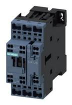
Power contactor, AC-3 25 A, 11 kW / 400 V 2 NO + 2 NC 220 V DC 4-pole size S0 Spring-type terminals 1 NO + 1 NC integrated
