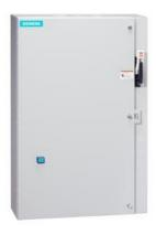
Non-reversing motor starter, Size 2 1/2, Three phase full voltage, Solidstate overload relay, OLR amp range 25-100A, 110V 50Hz / 120V 60Hz coil, Combination type, 100A circuit breaker, Enclosure NEMA type 1, Indoor general purpose use, Extra-wide enclosure
