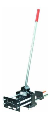
The TS-PSS 2 DIN rail cutter and punching tool is designed for manually shortening and punching holes in DIN rails (TS 15, TS 35, TS 32) and busbars (10 x 3 mm). The tool can be mounted on a workbench or similar working surface. It can also punch holes of varying dimensions in customized positions. A cross-hole/slotted-hole punch (12 x 6.4 mm) is included in the delivery.
