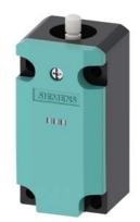
Basic switch for position switch 3SE5132 Plastic enclosure 40 mm according to EN 50041 Device connection 1 x (M20 x 1.5) with 2 LEDs, yellow/green, 24 V DC 230 V AC 1 NO/2 NC slow-action contacts without actuator head
