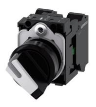
Selector switch, illuminable, 22 mm, round, plastic, white, selector switch, short, 2 switch positions O-I, latching, 10:30h/13:30h, with holder, 1 NO, 1 NC, spring-type terminal, with laser labeling, inscription or symbol Customer-specific selection with SIRIUS ACT configurator (CIN)
