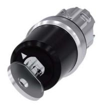
key-operated switch Siemens, 22 mm, round, metal, shiny, lock number SSG10, with 2 keys, 2 switch positions O-I, latching, actuating angle 90°, 10:30h/13:30h, key removal O+I
