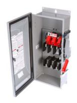
Siemens Low Voltage Circuit Protection Heavy Duty Safety Switches. Type: ENCLOSED, SAFETY SWITCH Std: CSA V. Rating: 240V A. Rating: 200A Wattage: 3W No. Of Poles: 3P F. Rating: 60Hz Action: SINGLE THROW Material: 304SS Enclosure: TYPE 12. 2-3 point mounting holes. Insulation: YES O. Cycles: 8000 O. Temperature: (-20F-120F) AMBIENT TEMPERATURE Environmental Conditions: INDUSTRIAL
