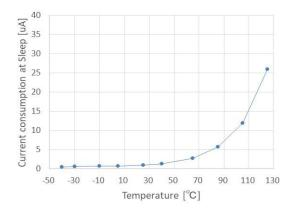
Fig.19 Current consumption at Sleep  $I_{\text{DDSL}}$ Temperature characteristics
