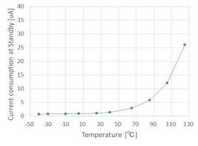
$\label{eq:consumption} \mbox{Fig.21 Current consumption at Standby $I_{\text{DDSB}}$} \\ \mbox{Temperature characteristics}$
