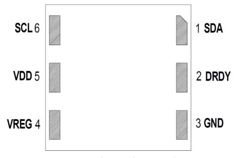
Fig.3 Pin configuration (Bottom view)
