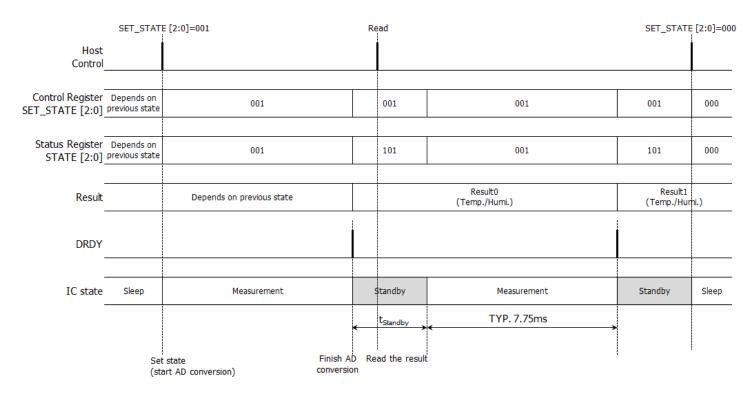
Fig.8 Timing chart for Repeat Operation
