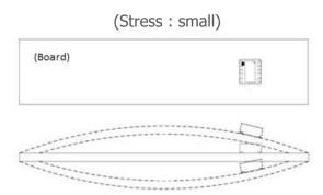
Figure C Mounting condition with less stress (Mounting position)
