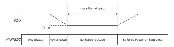
Fig. 5 Reapply voltage Sequence
