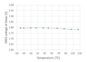
Fig.26 VREG voltage  $V_{\text{RGSL}}$ Temperature characteristics
