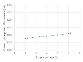
Fig.21 Current consumption at Measurement  $I_{\text{DDM}}$ Supply voltage characteristics
