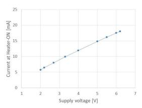
Fig.23 Current at Heater-ON I<sub>HEAT</sub> Supply voltage characteristics
