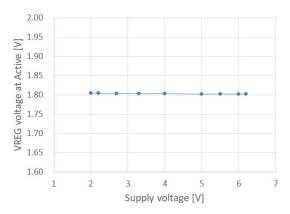
Fig.27 VREG voltage V<sub>RGACT</sub> Supply voltage characteristics
