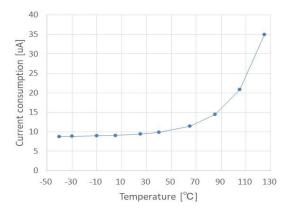
$\begin{array}{c} \text{Fig.17 Current consumption } I_{\text{DD}} \\ \text{Temperature characteristics} \end{array}$
