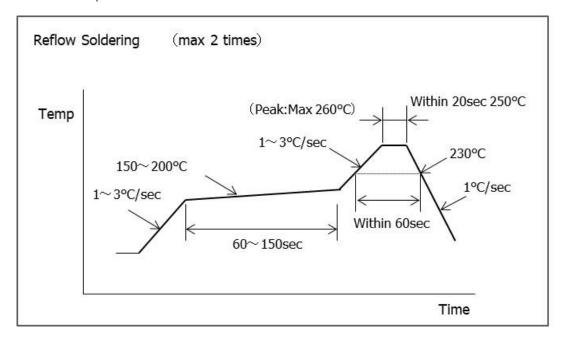
This profile gives recommended values, which are not guaranteed. For mounting the package, evaluate the profile with the equipment, conditions, and materials to be used.
