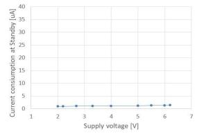
Fig.20 Current consumption at Standby  $I_{\text{DDSB}}$  Supply voltage characteristics
