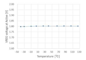
Fig.28 VREG voltage  $V_{\text{RGACT}}$  Temperature characteristics
