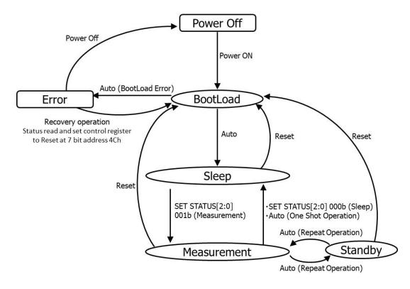
Fig. 10 State transition diagram
