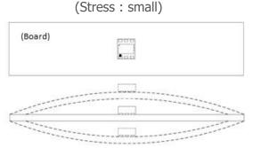
Figure B Mounting condition with less stress (Mounting direction)
