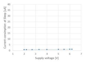
$\label{eq:consumption} \begin{tabular}{l} Fig. 18 Current consumption at Sleep $I_{DDSL}$ \\ Supply voltage characteristics \\ \end{tabular}$
