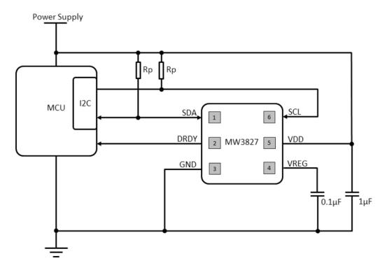
Fig.15 Typical electrical connection
