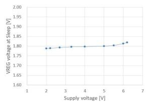
Fig.25 VREG voltage at Sleep V<sub>RGSL</sub> Supply voltage characteristics
