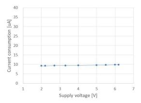
Fig.16 Current consumption  $I_{\text{DD}}$  Supply voltage characteristics
