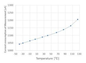
Fig.22 Current consumption at Measurement  $I_{\text{DDM}}$ Temperature characteristics
