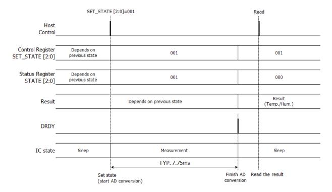
Fig.9 Timing chart for One Shot Operation
