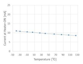
Fig.24 Current at Heater-ON I<sub>HEAT</sub> Temperature characteristics
