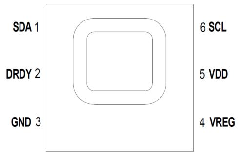
Fig.2 Pin configuration (Top view)
