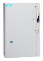
Non-reversing motor starter, Size 2 1/2, Three phase full voltage, Solid-state overload relay, OLR amp range 25-100A, Combination type, 100A circuit breaker, Enclosure NEMA type 1, Indoor general purpose use, Extrawide enclosure
