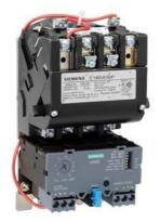
Non-reversing motor starter Size 1 Single phase full voltage Solid-state overload relay OLRelay amp range 3-12A 110VAC 50HZ / 120VAC 60HZ coil Combination type No enclosure
