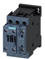
Power contactor, AC-3 38 A, 18.5 kW / 400 V 1 NO + 1 NC, 42 V AC 50/60 Hz, 3-pole Size S0, India 40 A, screw terminals
