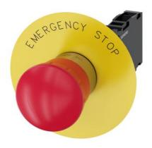
EMERGENCY STOP mushroom pushbutton, 22 mm, round, metal, shiny, red, 40 mm, positive latching, acc. to EN ISO 13850, rotate-to-unlatch, with yellow backing plate, inscription: EMERGENCY STOP, with holder, 1 NO+1 NC, screw terminal, Z=20-unit packaging
