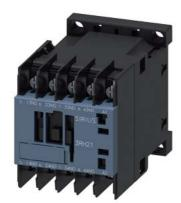
Contactor relay, 4 NO, 400 V AC, 50 Hz, 400 .. 440 V, 60 Hz, Size S00, ring cable lug connection
