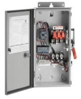
Slim Line Pump Control Panel NEMA size 1 Three phase full voltage Solid-state overload relay OLR amp range 10-40A 220/230V 50/60Hz Coil 30A fusible disconnect 30A/250V fuse clip 1NC / 1NO auxiliary contacts HOA Sel. Sw. <(>&<)> Start/Stop 3-point power terminal block 3-point control terminal block 3-point ground lug Enclosure NEMA type 3/3R Weather proof outdoor use
