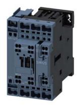
Contactor, AC-1, 35 A/400 V/40 °C, S0, 4-pole, 110 V AC, 50/60 Hz, 1 NO+1 NC, Spring-type terminal
