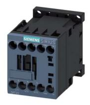
Power contactor, AC-3 9 A, 4 kW / 400 V 1 NO, 110 V AC, 50/60 Hz 3-pole, Size S00 screw terminal
