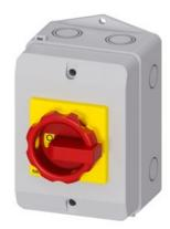
SENTRON, Switch disconnector 3LD, emergency switching-off switch, 3pole, Iu: 32 A, operating power / at AC-23 A 400 V: 11.5 kW, molded-plastic encapsulation for inch cable gland, 1 NC, 1 NO, rotary operating mechanism, red/yellow
