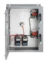
Duplex starter with alternator Size 0 Three phase full voltage Solid-state overload relay OLR amp range 0.75-3.4A 110VAC 50Hz / 120VAC 60Hz Coil Combination type Two 30A disconnect switches Enclosure NEMA type 1 Indoor general purpose use
