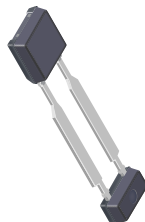
2-Pin SIP (suffix UB)
